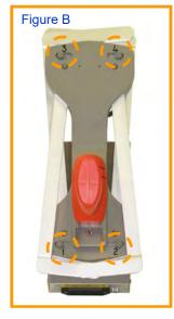
The directional antenna can be used in two ways. The R-300A receiver can be mounted on the FA-3 antenna for one handed operation or the CA-4 coax assembly can be attached so that the antenna and receiver can be separated.
